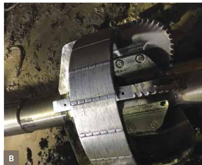
A-B: Hard Metal's first HDD tool, the Wombat Hole Opener, at work.
