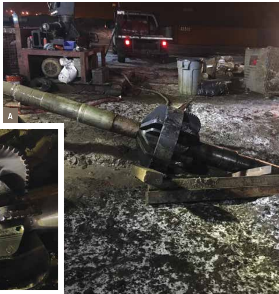
A-B: Hard Metal's first HDD tool, the Wombat Hole Opener, at work.
