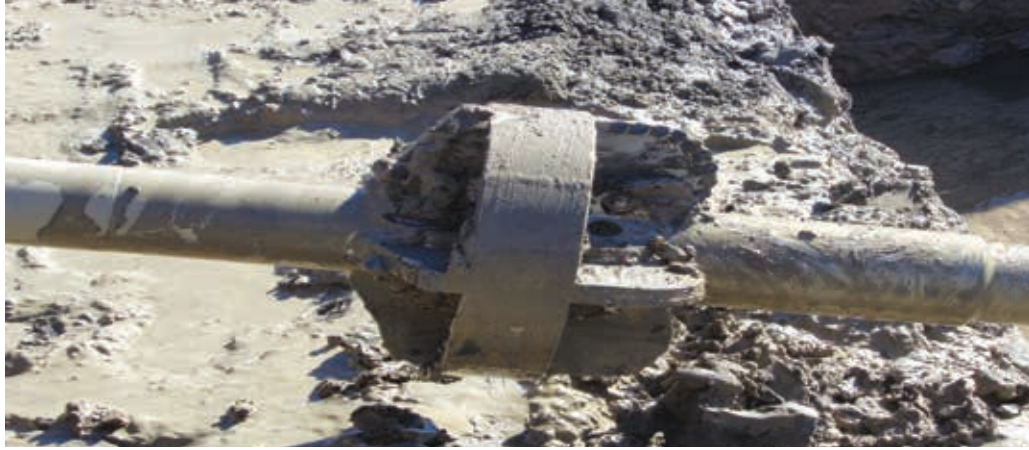
The Wombat hole opener features changeable cutter wings, a stabilizing ring, and a Nord-lock washer, the same locking system used by NASA.
