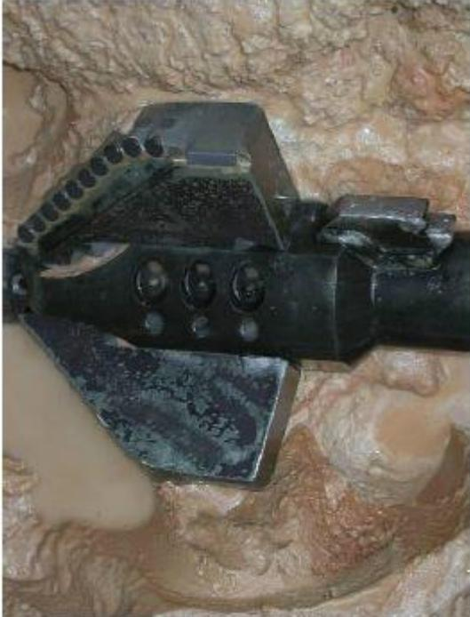
**The first development step was to use field-replaceable cutter wings.**
