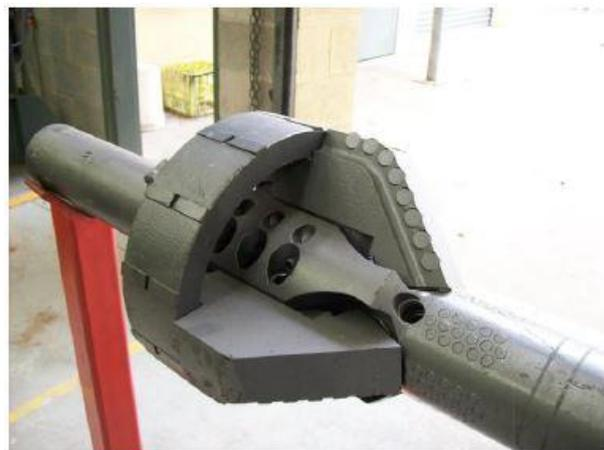
**The next version incorporated a stabilisation ring to locate the cutter wings more securely.**
