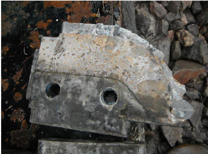
however the conditions in the bore were highly unfavourable and it was decided to use less expensive Tungsten Carbide Cutting Wings (Fig 8) through these sections as sacrificial cutters until the bore progressed into more favourable mudstones and sandstones.
