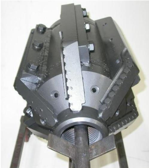
The series 3 (Fig 6) discarded weight but was more robust in design. It was more easily field serviced and delivered excellent ROP. On one particular site, the ROP was in excess of 30 metres/hour. Still it suffered from insufficient stabilisation and as a consequence, PDC life was short and service costs were higher than anticipated.
